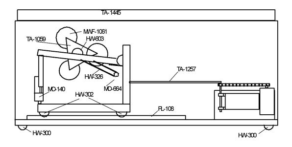
TA-1445 - Complete Top Oushion Assembly HW300 - Ball Caster HW302 - Rgid Caster PL-108 - Caster Track TA-1257 - Rush Arm MD-140 - Height Actuator MWF-1061 - Massage Roller TA-1059 - Traingle Assembly HW4603 - Triangle Assembly HW4603 - Triangle Pillow Block Bearing MD-664 - Roller Motor HW326 - 76 Rtch Roller Chain
