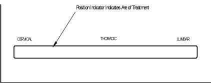
TREATING A SPECIFIC AREA-When position indicator reaches desired area, turn travel switch off. An eight (8) inch area will be continually treated
